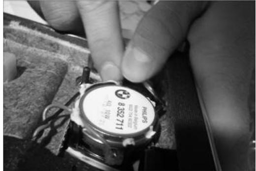
**2.** Place the new tweeter over the location where the factory tweeter was located and apply several dabs of the included adhesive around the outer perimeter.
