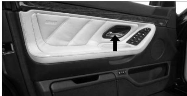
**2.** Remove the Philips head screw. This may also be a Torx T20.
