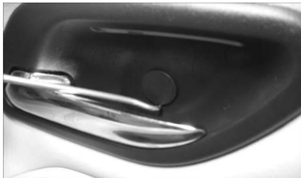
**3.** Now, CAREFULLY pry out the window controls using a small, flat head screwdriver.
