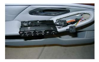
**4.** We now need to remove the light on the underside of the door panel. Using your panel removal tool, pop the light out by prying on the inner and outer edges of the light. It will just pop out, at which point you'll simply unplug the light. This can be a bit trying, but once you figure out the first one, the other doors will be a breeze.
