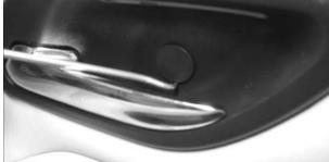
**3.** Now, CAREFULLY pry out the window controls using a small, flat head screwdriver.
