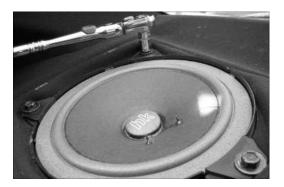
5. Simply slide the terminals attached to the new speaker into the existing factory plugs in the same way as the front speakers.
