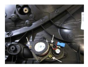
**2.** You'll simply reattach the new midrange/ tweeter housing into place using the factory hardware that was removed from the factory speaker housing.
