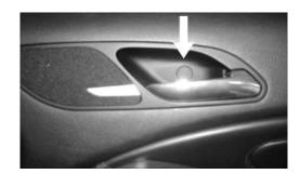
**7.** Carefully insert your panel removal tool on the front side bottom edge as shown. Pry steadily outward until your hear the clip(s) release themselves.
