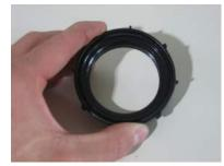
**8.** Drop the new midrange into the ring and place a few dabs of the included adhesive around the speaker securing it to the ring. Let the adhesive cure for at least an hour before reinstalling.
