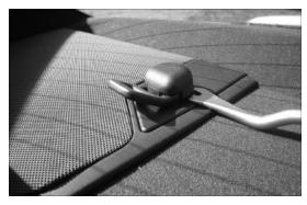
2. This will reveal a 13mm bolt. Remove this using your socket wrench
