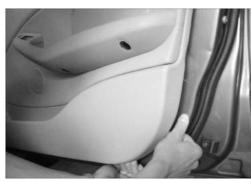
**9.** Carefully pull outward and upward from the rear of the door along the top edge to fully release the panel.
