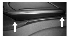
**4.** Locate the airbag plug towards the rear center of the door panel. Remove this using your panel popper. Pry from the top and bottom very carefully. This will reveal another Torx T20.
