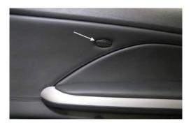
**5.** You will also need to pop out the side mirror control switch in the driver's door. Remove it using a small flat head screwdriver, lifting upward from the rear of the switch, and unplug. This may also be done when the door panel is off by using your finger to push it out from the inside.
