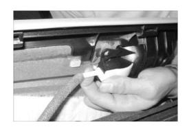
**11.** Unplug the speaker wires from each speaker and the panel can now be removed.
