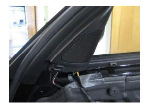
**2.** Use your plastic panel removal tool and carefully pry at the location of the arrow. Once the plastic housing is free, it will free itself and allow you to gain access to the tweeter.
