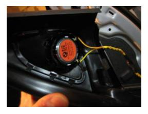
**IMPORTANT!** Before installing your new BAVSOUND tweeter, you **MUST** plug the included capacitor harness inline with the front tweeter or your tweeter will **NOT** function correctly.
