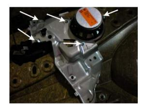
**2.** With the speaker removed, we can now apply the optional sound deadening material to the door panel itself. (Optional: start by heating the sound deadening up to activate the glue on the sticky side of the material).
