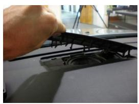
**2.** The speaker is held in either by (3) 8mm bolts, or in some cases, Philips head screws.
