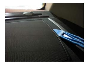
**3.** Once the front clips release, remove the cover by lifting upward slightly and sliding the cover towards the front of the car.
