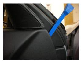
**5.** The door panel is secured by a large plastic clip located roughly in the middle of the door panel.
