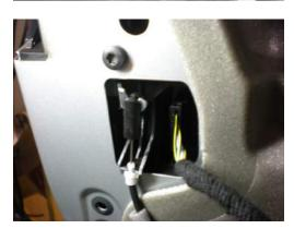
**8.** Completely remove the wiring harness that runs along the upper section by using our panel removal tool and freeing the plastic fasteners that secure it to the door.
