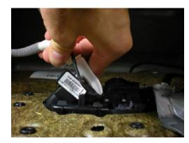
10. We can now disconnect the window switch and free the harness gong down to the light, thus allowing us to work on the panel. The rest of the installation must take place with the panel on our laps, as the panel cannot be completely removed due to the airbag.
