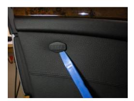
**4.** Now, we need to locate the small screw cover on the front inside edge of the panel. Using your angled pick tool, carefully remove the cover as shown. You may pierce the plastic with your tool, but don't worry. There is a Philips head screw behind this cover. Remove it and place it aside.
