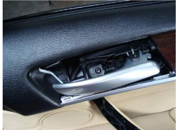
**5.** Again, using your plastic panel removal tool, carefully pry along the bottom edge of the door pull, as we're going to separate the front of the pull from the rear.
