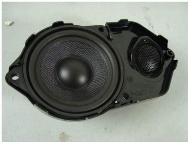
4. Head back over to the X5, and plug the midrange into the factory connector. Reattach the housing, snap the grille back in, and pat yourself on the back.
