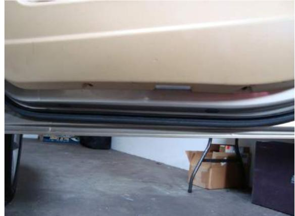
**2.** Now is also a good time to pop out the light on the underside of the panel as well. Using your plastic panel removal tool, carefully pry out the front edge (closest to the front of the car when the door is closed). The light will pop out, and you can unplug it. Place this aside in the area where you will also be keeping the screws.
