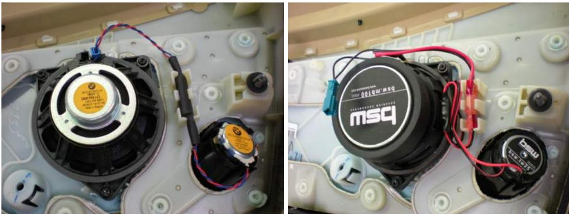
**IMPORTANT!** Before installing your new BAVSOUND tweeter, you **MUST** plug the included capacitor harness inline with the front tweeter or your tweeter **will NOT** function correctly.
