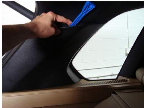
**2.** With the panel removed, detach the midrange/tweeter pod by removing the three Philips head screws that attach it to the body.
