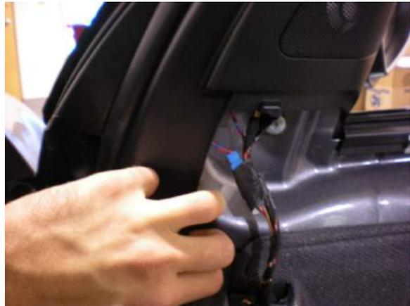
**2.** With the front edge loose, push toward the rear of the door, freeing the rear lip of the tweeter panel.
