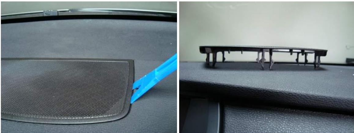
2. The midrange/tweeter housing is attached using 4 Torx T20 screws. Remove these, unplug the assembly, and take the pod to your workstation.
