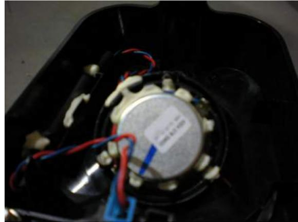
**IMPORTANT!** Before installing your new BAVSOUND tweeter, you **MUST** plug the included capacitor harness inline with the front tweeter or your tweeter **will NOT** function correctly.
