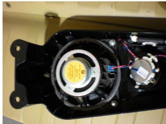
**3.** Take the pod to your workspace. Remove the three 8mm nuts that attach the factory midrange.
