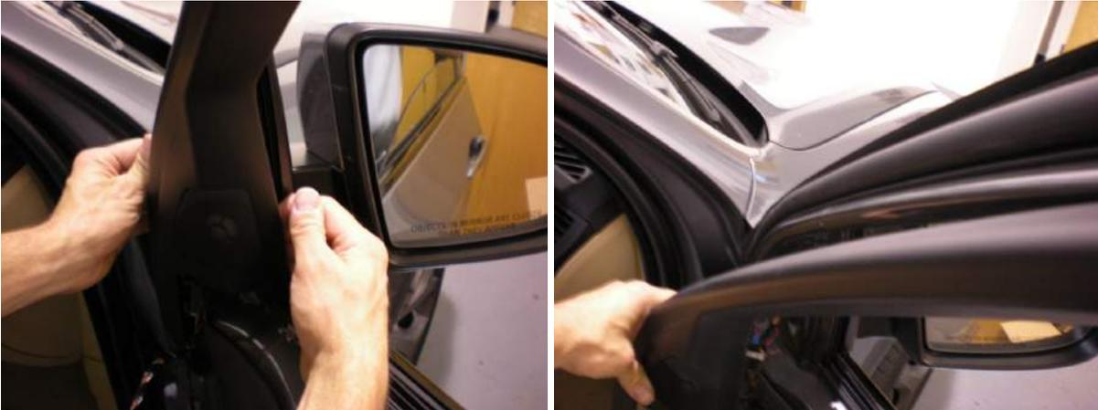
**4.** Pry off the foam, and with the factory tweeter exposed, remove it using your angle pick tool. Carefully pry out at the attachment points, and the tweeter will free itself.
