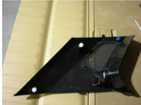
**1.** Using your panel removal tool, carefully pry out the rear D Pillar starting at the top edge. Use your hands to remove the panel.
