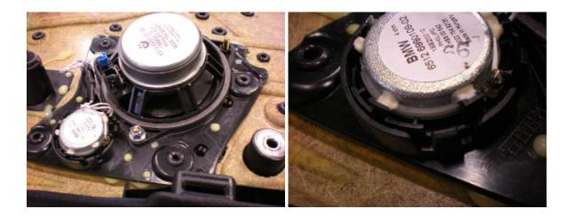
9. As you can see, we'll need to carefully pry the factory tweeter out of it's housing. Using your right-angle pick tool, carefully pry the tweeter out by prying the three attachment points outward and lifting upward with your pick tool.
