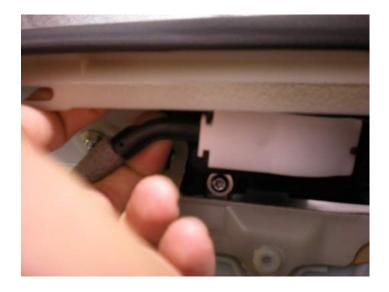
8. With the panel free, take it to your workspace and prepare for the midrange installation. The midrange is attached using three 8mm nuts. Remove these, and unplug the tweeter connector from the midrange.
