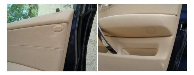
2. Next, we'll remove the woodgrain (or aluminum, depending on your interior trim) panel that covers the door handle. There are two more Torx T25 bolts behind this panel, both of which will need to be removed.
