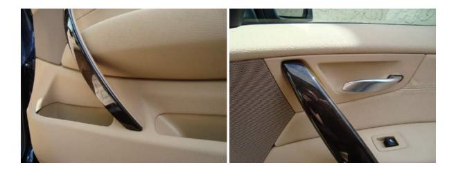
3. With the cover and bolts removed, we can now remove the panel itself. Using your plastic panel removal tool, carefully pry the door panel starting along the edge at the upper left of the panel, shown here.
