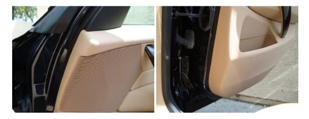
6. The picture on the right shows you the blue "clips" that you'll be removing. Once that top left corner is removed, begin working your way around the panel until it is completely free. Take a firm grip while pulling in towards the car. The top edge is going to require a small amount of finesse, which you'll see as you get there. Don't force anything. It will come off, we promise.
