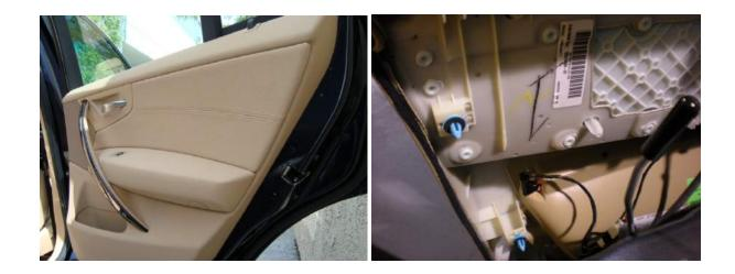
7. With the panel now free, the first thing we'll do is unplug the speakers, window controls and lighting. Simply pull outward away from the speaker/switch, and the connectors will free themselves. Now, we need to pop out the door latch mechanism. It's easy, don't worry! Just place your fingers behind the switch as shown, and pull away from the panel:
